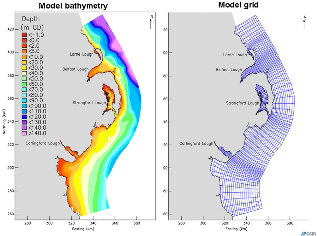
Fig. 3. Delft3D model bathymetry and grid. Note the very dense grid inside the lagoons, comprising hundreds of cells and 8 sigma layers.
