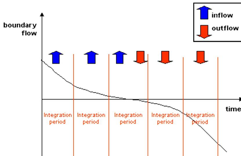
Fig. 4. Flow integration for EcoWin2000, illustrating the need for bidirectional flows (courtesy J.P. Nunes).
